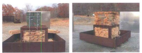
Figure 7. External Fire/Fast Cook-Off Test Setup
